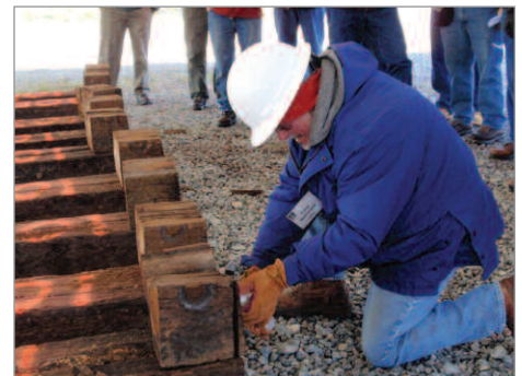
Amburgey sprays color test reagent on sectioned ties.
